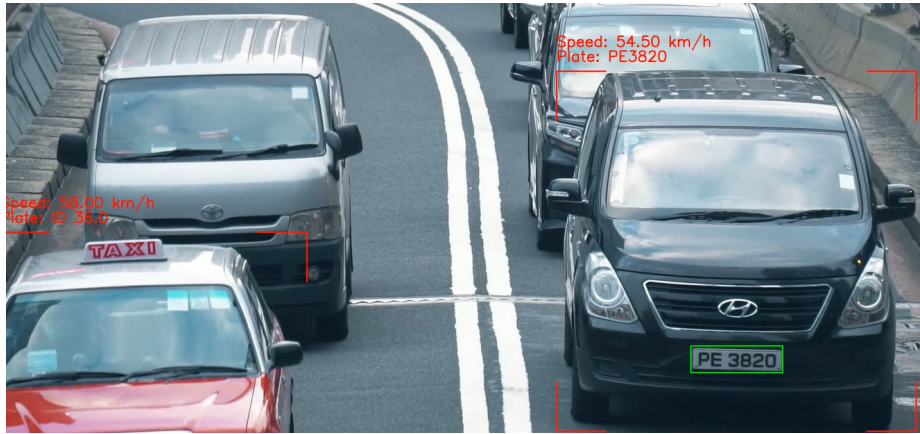
Fig. 4: Speed estimation and license plate recognition using YOLOv11, SORT, and EasyOCR.
